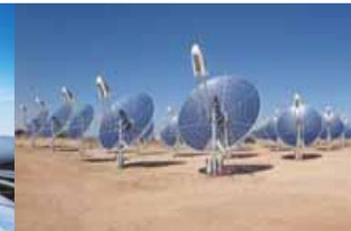
Parabolic dishes with Stirling motors
