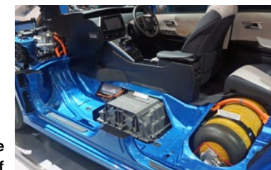
Toyota Mirai Fuel Cell cutaway
